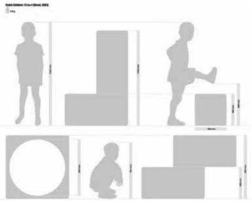
The shape of the Blocks is derived from Tetris blocks i.e. T-shape, L-shape, square-shape and Z-shape. The measurements of the Blocks can be seen in the image above and are based on the measurements of 12-year-old children. The weight of a Block is +-380 kg which makes them sturdy to play on.
